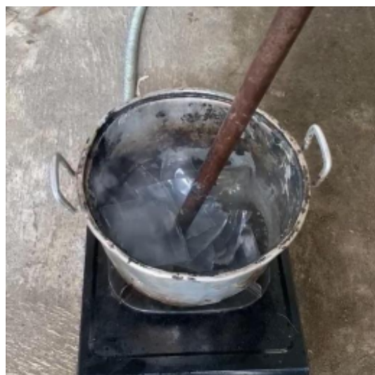
Gambar 5 . Proses pelelehan plastik
