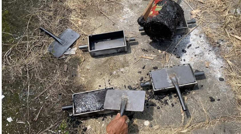
Gambar 2 Proses Percetakan Paving Block
